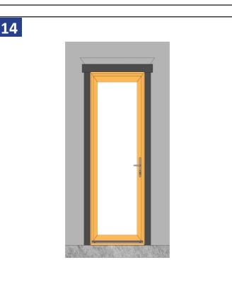
Cut a piece of flashing tape for the head flashing, which extends beyond outer edges of jamb flashings. Remove release paper and adhere to exposed sheeting or framing members.
