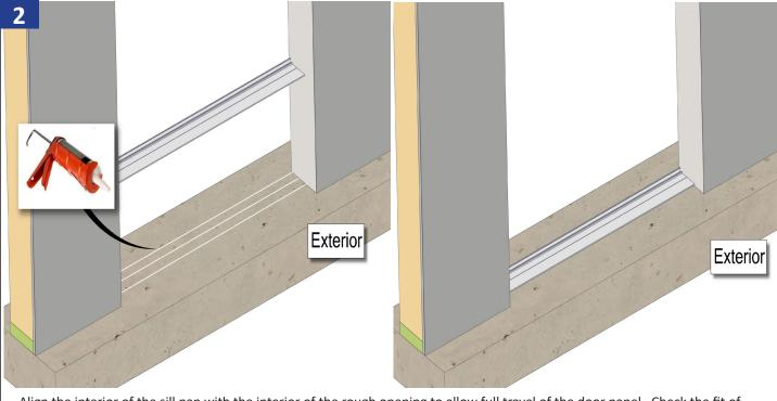
Align the interior of the sill pan with the interior of the rough opening to allow full travel of the door panel. Check the fit of the sill pan system making sure the conditions are level. Apply three 3/8" continuous beads of silicone across the entire width of the rough opening threshold. **THRESHOLD MUST BE LEVEL!** Quaker recommends **self-leveling concrete**, if not available - shim 12" or less on center.
