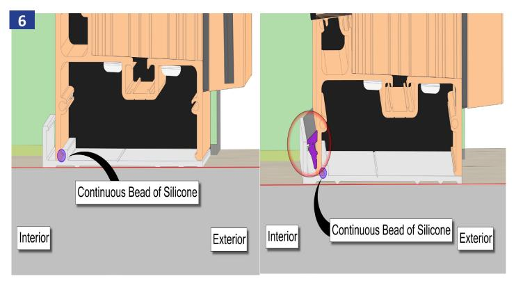
Set door position shown above. Once the door has been set on the sill pan, install the wedge gasket (circled).
