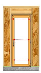
Press the backer rod (blue) into the space between the building condition and the frame. Then apply a continuous bead of sealant (red) in the same space over the positioned backer rod, tool in sealant. Ensure that the space between the frame and the building condition is completely sealed.
