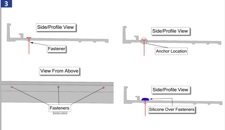
After placing sill pan, pre-drill holes and fasten the sill pan in place with screws per shop drawings or anchorage calculations. Typically #8 x 2" deck screws that are 4" from each end and 14" on center at the threshold. Ensure that every fastener location is sealed generously and completely with silicone.
