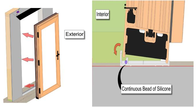
Center and set the door frame into the rough opening, making sure there are equal gaps on both sides of the door frame. Angle the door frame with the top tilted out, and set the door threshold onto the sill pan so the notches meet at the continuous bead of silicone.
