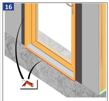
Install and fasten the door unit in place using fasteners by others per anchorage calculations. Always follow the anchorage calculations and fastener/anchor manufacture's guidelines for proper edge distance, load capacity and installation techniques.
